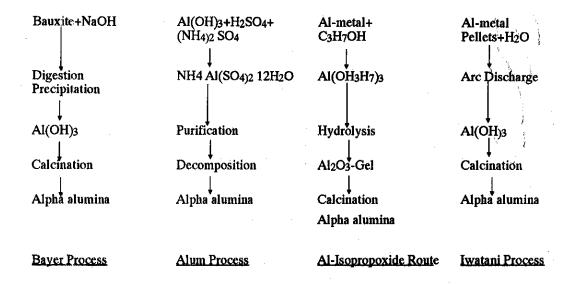
The Bayer Process produces a wide range of aluminas, some of which have Na<sub>2</sub>O levels well below 0.01 wt% and varying grain sizes corresponding to specific surface areas of 0.5 to 20 m<sup>2</sup>/g BET. Aluminas with lower values of Na<sub>2</sub>O are produced via the alum process, the Itawani process or by the hydrolysis of aluminium oxides.
